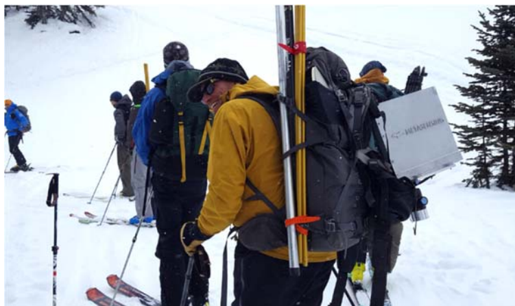
Figure 18: Square trihedral corner reflector being deployed on the field by ground team.
