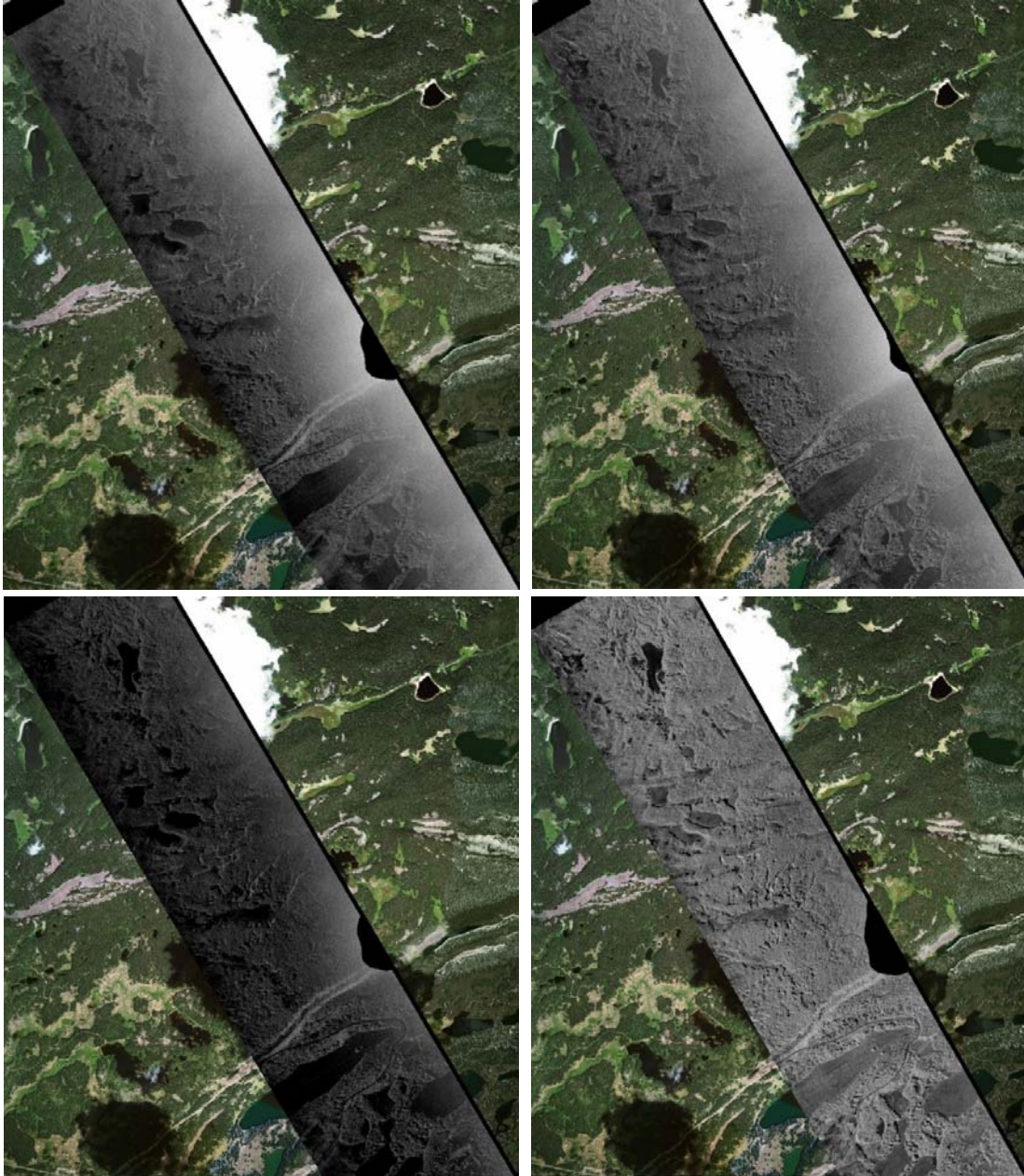
Figure 13 - SnowSAR images at X band, relatively to the track 20170221202338. From top left, clockwise: HV, HH, VV, VH polarizations. Geotiff format, intensity values scaled from -30 to 0 dB.
