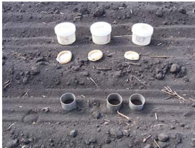
Figure 29. Aluminum sampling rings ready to be inserted alongside a hydra probe reading location. Sample containers are for transporting each sample to the lab for weighing.
