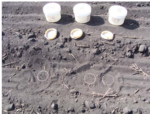
Figure 31. Aluminum sampling rings fully inserted alongside a hydraprobe reading location
