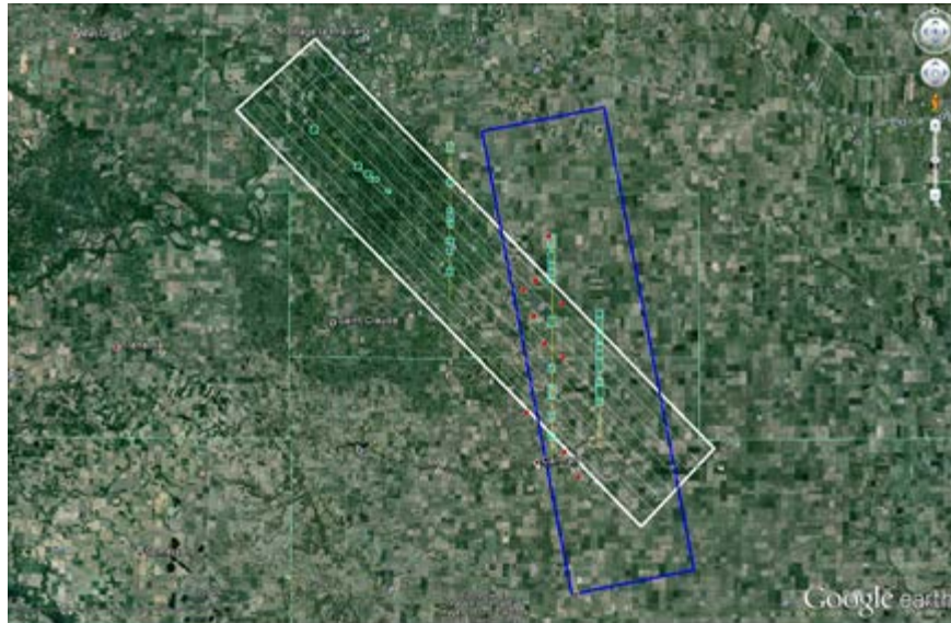
Figure 23. TerraSAR-X ascending pass over the SMAPVEX site. Acquisitions will be around 6:00 PM (local time) at an incidence angle of around 30°
