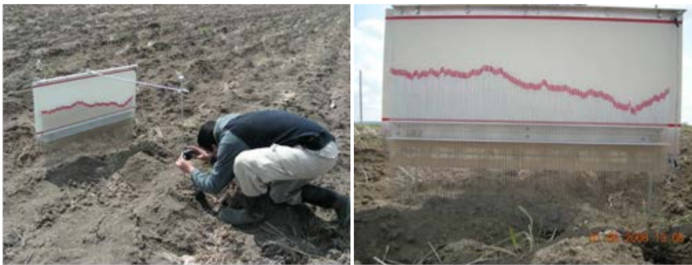
Figure 17. Capturing surface roughness with the roughness profilometer.
