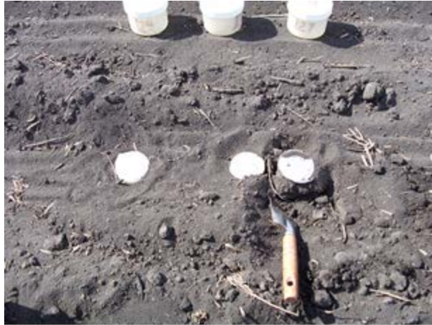
Figure 32. Loosening a sample ring to remove the sample from the soil
