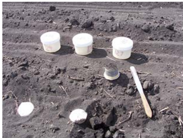
Figure 33. A sample that has been trimmed to size and now ready to be transferred to the sample container
